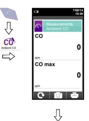
Connect the gas probe to the instrument and perform the measurement. Wait 5 minutes.
